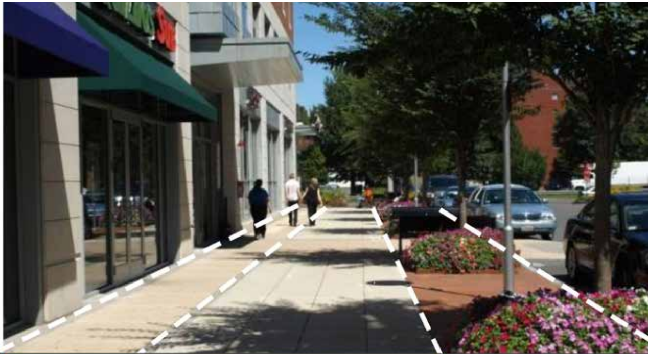
BUILDING DISPLAY, BENCHES, ETC. PATH OF PEDESTRIAN TRAVEL TREES, PLANTERS & LIGHT POLES ON-STREET PARKING
